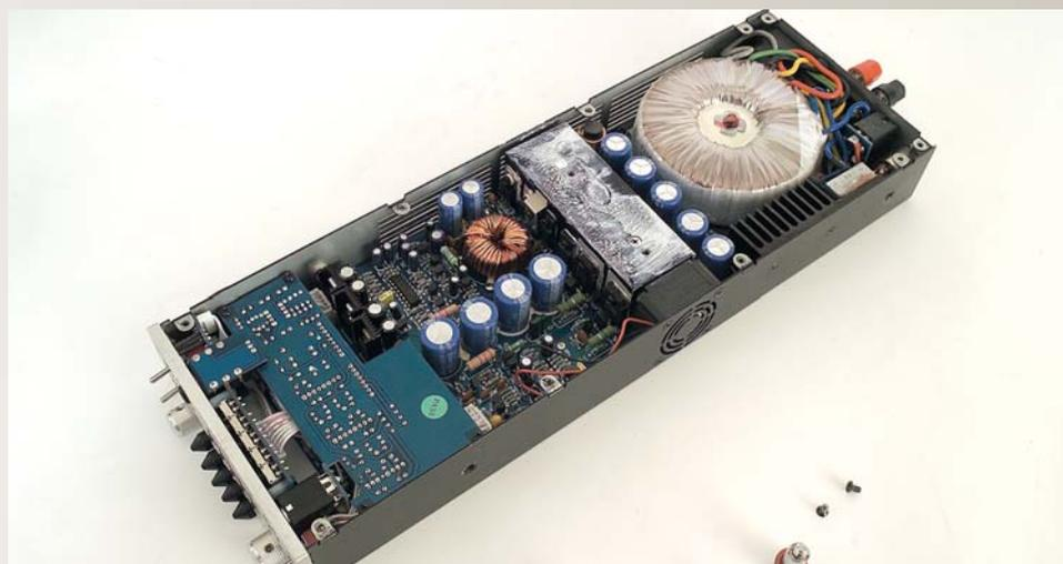
The Briefcase's interior is a model of space efficiency. Note the heatsink tunnel and fan, which separates the sensitive preamp components from the power supply at the rear.
